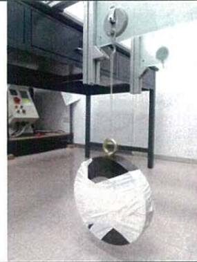
Photo "B" Static Load Test: 9430080
